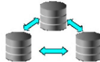
Peer-to-Peer Load Balancing, Multimaster
